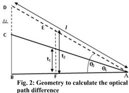
The value of  $\left(\frac{\Delta\theta}{\Delta T}\right)$  can be found by plotting a graph for  $\theta \sim T$ . Typical values of  $\alpha$  for aluminium, copper and brass at room temperature are 23.1 × 10<sup>-6</sup>, 16.6 × 10<sup>-6</sup> K<sup>-1</sup> and 20.3 × 10<sup>-6</sup> K<sup>-1</sup>, respectively
